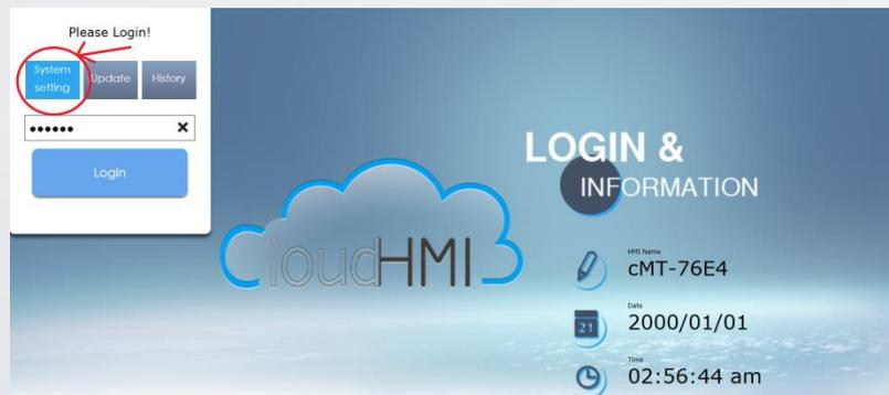
**Step 8.** After login, the page will lead you to the setting page of Network. You can choose whether to set the IP of Ethernet 1 or Ethernet 2 as DHCP or Static IP.
