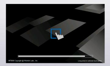
Step 3. Touch the center of all the "+" signs on the screen with your finger or a stylus. The signs disappear if correctly touched, and the touch parameters are stored in the system.
