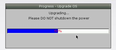
**Step 9.** When finish upgrading, the system will restart HMI. After this, touchscreen calibration is highly recommended.
