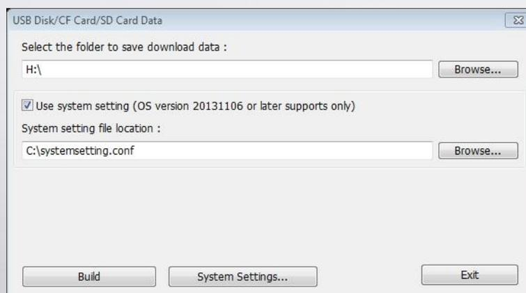
**Step 5.** Click [Build] button to generate the file for download by using USB drive or SD card. A “config” folder can be found as shown below.
