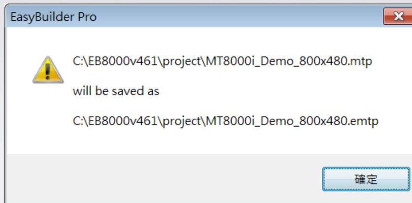
**Step 7.** EBPro V1.11 will save mtp file as emtp file, which is different from EB8000 mtp file for distinguishing.
