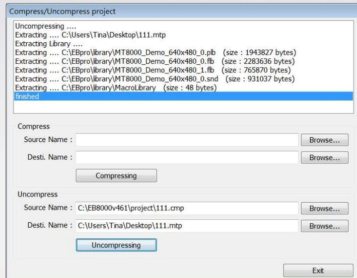
**Step 5.** Open the mtp file gained from uncompressing, EBPro will show System Parameter Settings window, in HMI model selection, select the eMT3000 type to be translated into, click OK.
