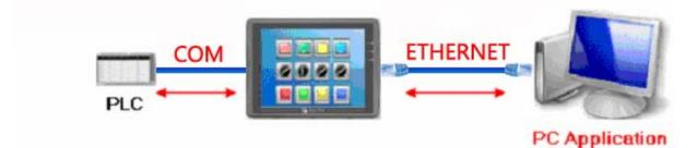
First, a virtual serial port must be created on PC. The application program on PC can communicate with PLC through this virtual serial port.
